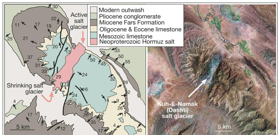
**Figure 2. Surface geology (left) and Landsat image (right) of Kuk-e-Namak (Dashti), Iran, 28°16'N, 51°42'E. Faults intersecting the anticlinal dome facilitated salt breakout and formation of surface salt glacier, or namakier. Black arrows indicate bedding dip and azimuth in anticlinal beds (geology after Kent, 1958; Landsat image courtesy of National Aeronautics and Space Administration).**
